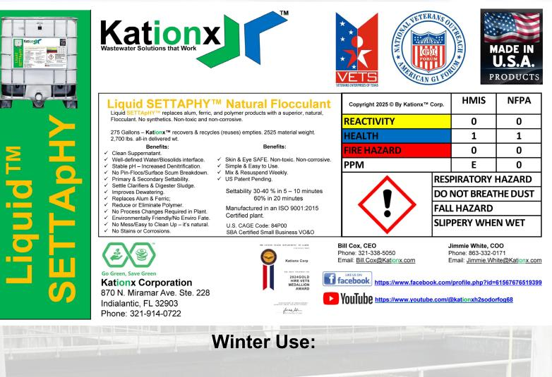
Keep Liquid SETTApHY<sup>™</sup> in emulsion to lower freezing point. In freezing temperatures mix every afternoon. To prevent an ice layer from forming store totes indoors.
