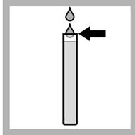
1. Fill the measuring tube with sample.
