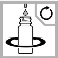
6. Add the Sulfuric Acid Standard Solution by drops. Mix after each drop. Count the drops until the color changes from green to pink.
