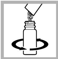
2. Add one Phenolphthalein Indicator Powder Pillow. Swirl to mix. If the solution is colorless, the Phenolphthalein (P) alkalinity is zero. Go to step 5.
