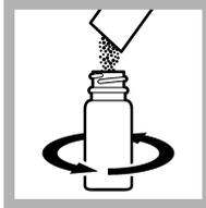
3. Add one Phenolphthalein Indicator Powder Pillow. Swirl to mix. If the solution is colorless, the Phenolphthalein (P) alkalinity is zero. Go to step 6.
