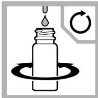
3. Add the Sulfuric Acid Standard Solution by drops. Mix after each drop. Count the drops until the color changes from pink to colorless.
