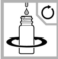
4. Add the Sulfuric Acid Standard Solution by drops. Mix after each drop. Count the drops until the color changes from pink to colorless.
