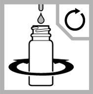
7. Add the Sulfuric Acid Standard Solution by drops. Mix after each drop. Count the drops until the color changes from green to pink.
