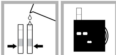
1. Fill two tubes to the first line (5 mL) with sample.
