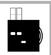
5. Put the second tube into the color comparator box.
