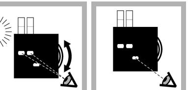
6. Hold the color comparator box in front of a light source. Turn the color disc to find the color match.
