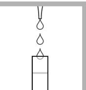
3. Add 8 drops of bromthymol blue pH indicator solution to the second tube.
