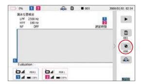
To listen to the sound of each pre-amplifier from the headphones connected to the main unit, tap the right edge of the correlation screen to display the quick menu.
