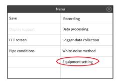
Press the main unit menu switch E. Tap "Equipment setting" under Menu.
