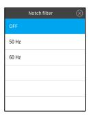
Select a notch filter from the following choices. OFF, 50 Hz, or 60 Hz
