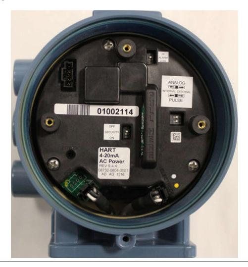
Figure 6-1: Electronics Stack and Hardware Switches
