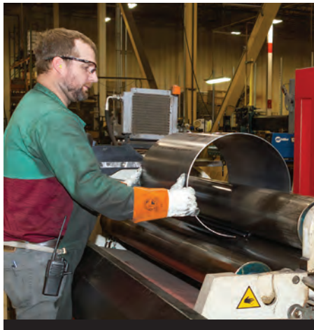
Automated CNC roll former rolls up to 3/16-inch steel to create the shell of an air compressor vessel.
