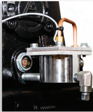
Low oil sensor does not allow unit to start when oil levels fall below an adequate level
