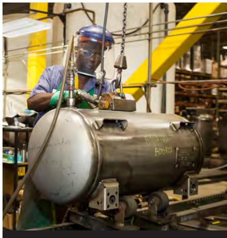
Advanced hydrostatic testing is performed on every air compressor vessel manufactured at Mi-T-M to verify leak-free construction.
