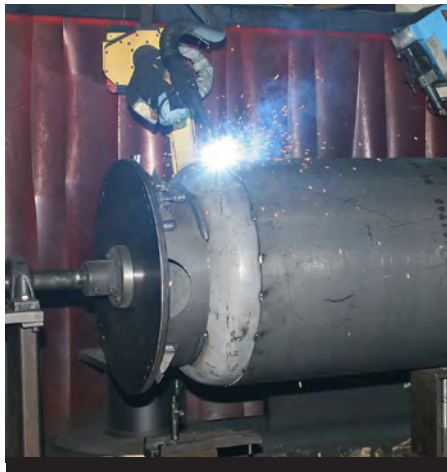
Of the 13 robotic welders at Mi-T-M, two are dedicated to welding air compressor vessels.
