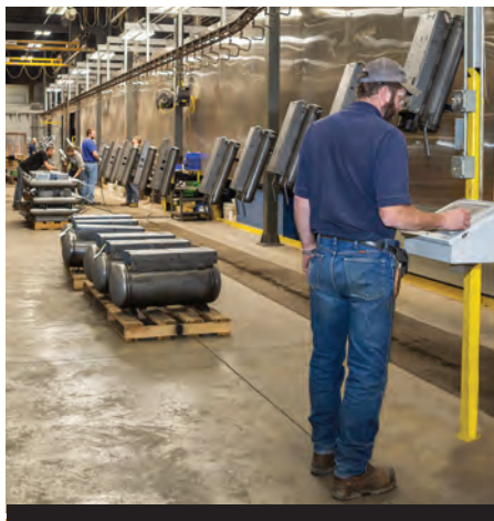
A 6-stage powder coated system applies superior finish that is harder and more durable than conventional paint.
