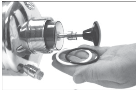
Step 5 – Remove Washer & O-Ring
