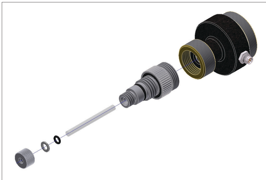
Figure 15 – Removing Quartz Rod from Remote Probe
