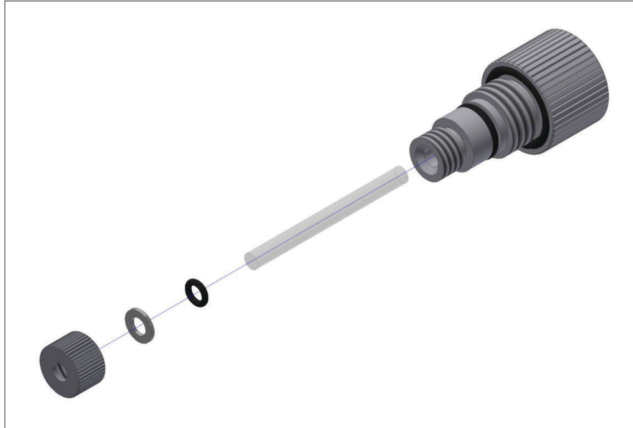
Figure 15 – Removing Quartz Rod from Remote Probe
