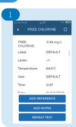
The first line displays the test type and the measured concentration (after dilution if applicable).
