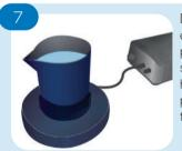
During the one minute electrochemical measurement period, set up the degasser as shown. Ensure the two plastic halves of the degasser are properly connected. Ensure the filter is installed correctly.
