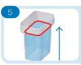
Fill the disposable vessel to the shoulder. Do not overfill, or water can splash onto the sensor contacts and interfere with the test.
