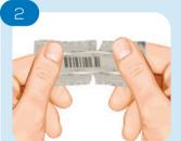
Tear each side of the packet, then twist and tear the short side from the packet, revealing the sensor tracks. Do not touch the dosed half of the sensor
