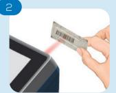
Scan the sensor barcode using the barcode scanner. Hold the barcode about 12cm (5 inches) from the instrument. Align the red dot with the center of the barcode. When the scan is complete, the instrument proceeds to the next screen.
