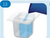
Fill the right side of the vessel to the line with degassed water.
