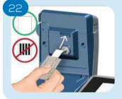
Hold the final CDX sensor through the foil packet only, with the white side facing up. Slide it all the way in, until the end stops against the back of the slot.
