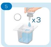
If chlorine or copper is present in the solution, add three drops of glycine reagent to prevent them from interfering with the measurement. Use the stir rod to mix the sample. If no chlorine or copper are present, skip this step.
