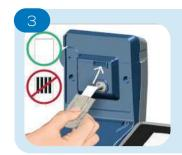
Hold the sensor through the foil packet only, with the white side facing up. Slide it all the way in, until the end stops against the back of the slot.
