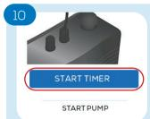
Press the START TIMER button to begin the timer. The displayed time is calculated based on the concentration of chlorine dioxide measured in the previous step.
