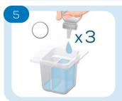
If chlorine or copper is present in the solution, add three drops of Glycine reagent to prevent them from interfering with the measurement. Use the stir rod to mix the sample. If no chlorine or copper are present, skip this step.
