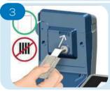
Hold the sensor through the foil packet only, with the white side facing up. Slide it all the way in, until the end stops against the back of the slot.
