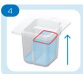
Fill the right side of the vessel to the line. If there is excess sample, it will pour into the left side of the vessel. Do not overfill both sides or water can splash onto the sensor contacts and interfere with the test.
