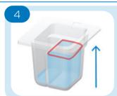
Fill the right side of the vessel to the line. If there is excess sample, it will pour into the left side of the vessel. Do not overfill both sides or water can splash onto the sensor contacts and interfere with the test
