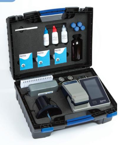
The chlorite test method involves three separate measurements of various chemical combinations in the sample, followed by some calculations to determine the total chlorite concentration. The test procedure must be followed carefully to ensure the chemical reactions and measurements occur correctly.
