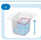
Fill the right side of the vessel to the line. If there is excess sample, it will pour into the left side of the vessel. Do not overfill both sides or water can splash onto the sensor contacts and interfere with the test.
