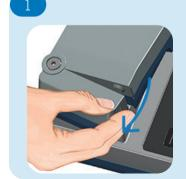
Open the front lid to drop the sensor into the disposable vessel.
