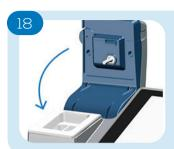
Close the arm with no sensor inserted.
