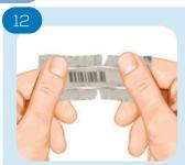
Tear each side of the second CDX sensor packet, then twist and tear the short side from the packet, revealing the sensor tracks. Do not touch the dosed half of the sensor.
