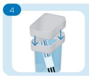
Place a cap on the disposable vessel. If required by local regulations, dispose of the sample, sensor and vessel in a secure manner.
