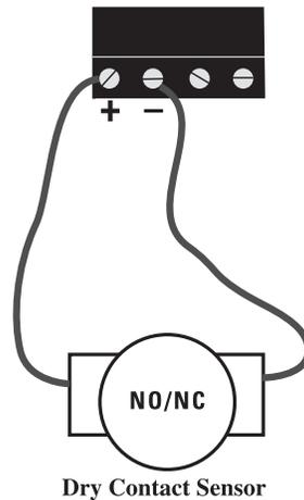
Wiring a Dry Contact Sensor
