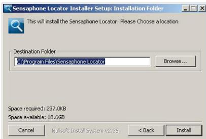
This dialog allows you to specify the location where the executable will be installed. When you are satisfied with this value, press the Install button.
