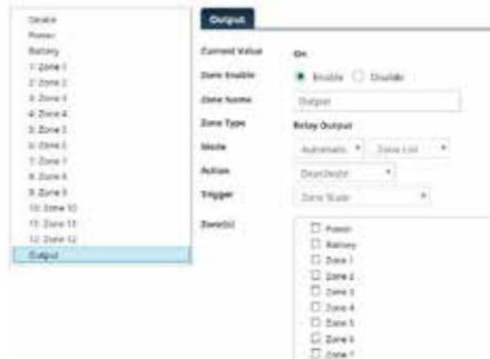
Enter a Name so that you'll know what the Output will be controlling. The Output can operate in Manual mode or Automatic mode. In manual mode you can turn the relay ON or OFF through the web page or the mobile App. To manually switch the relay output, click in the State field and select either ON or OFF, then click *Save Changes*. The change request will be sent to the Sentinel and the *Current Value* will update after the output change has successfully completed.
