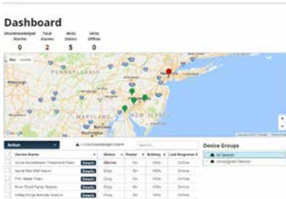
The device table will display all devices on your account. Click on the *Details* button to display and configure the zones for that device. You can also use the search box above the table to search through the table, or click on the table column headers to sort the data.
