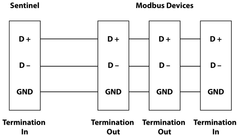
Connect the ground terminal (GND) on the Sentinel Pro RS485 terminal strip to the corresponding ground or shield terminal on the Modbus slave device. Connect the Sentinel Pro RS485 Transmit/Receive Positive (D+) terminal to the corresponding positive data terminal on the Modbus slave device. Connect the Sentinel Pro Negative (D-) terminal to the corresponding negative data terminal.
