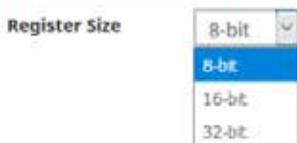
**Register Size:** Specifies the size (in bits) of each register that the slave device is sending to your Sentinel Pro. A register size of 16 bits is the de-facto standard however the Sentinel Pro will also support registers of 8 and 32 bits in size.
