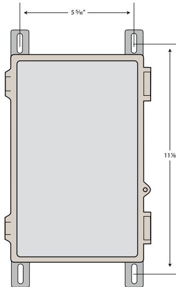
Figure 1: Mounting Dimensions
