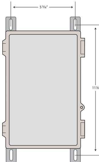
Figure 1: Mounting Dimensions
