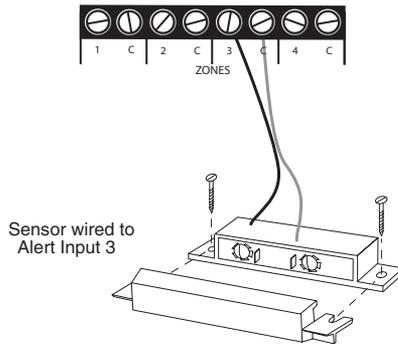
Figure 2-6. Sensor Connected to an Alert Zone
