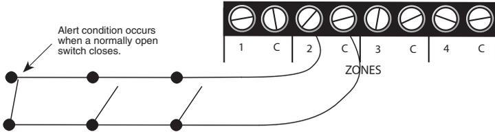
Figure 2-9 Multiple Normally Open Sensors
