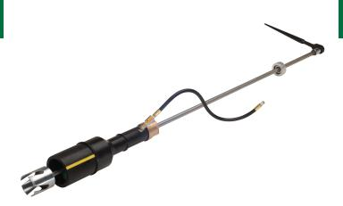
Tap live mains without service disruptions with McElroy's Hot Tap Tools for polyethylene pipe in both imperial and metric sizes. The Hot Tap Tools make it possible to add new service connections to live mains while keeping existing services up and running. They provide the most precise and economical way to tap through 2", 3", 4" and 6" branch saddles. The gland is customized to meet the user's material of choice, eliminating the need for material compatibility fusion in the field.
