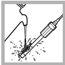
2. Rinse the probe with deionized water. Dry the probe with a lint-free cloth.
