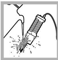
3. Rinse the probe with deionized water. Dry the probe with a lint-free cloth.
