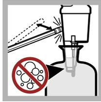
**6.** Tap the probe to remove air bubbles.
