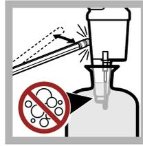
3. Tap the probe to remove air bubbles.
