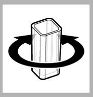
4. Turn the sample cell left and right to mix.
