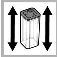
3. Put the cap on the sample cell. Shake the sample cell for 15 seconds.
