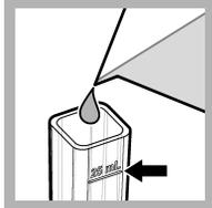
1. Fill the sample cell to the 25-mL mark with sample.
