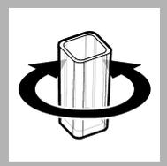
6. Turn the sample cell left and right to mix.
