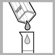
6. Remove the cap. Pour the solution into the graduated cylinder.
