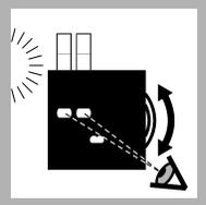
6. Hold the color comparator box in front of a light source. Turn the color disc to find the color match.
