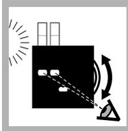
7. Hold the color comparator box in front of a light source. Turn the color disc to find the color match.
