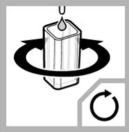
5. Add the Sulfuric Acid Standard Solution by drops. Mix after each drop. Count the drops until the color changes from green to pink.
