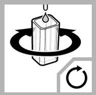
7. Add the EDTA Titrant Solution by drops. Mix after each drop. Count the drops until the color changes from pink to blue.
