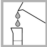
1. Fill the graduated cylinder to the 23-mL mark with sample.
