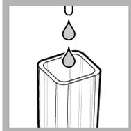
3. Add two drops of the 8 N Potassium Hydroxide Solution.
