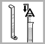
7. Look in the graduated cylinder from the top. Slowly put the cyanuric acid dipstick into the cylinder until the black dot is not seen.
