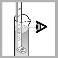
8. Look at the scale on the dipstick. The number on the dipstick scale at the surface of the solution is the result in mg/L.
