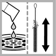
9. Discard the solution. Clean the sample cell and graduated cylinder with soap and a brush.
