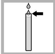
1. Fill the measuring tube with sample.
