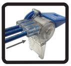
Insert striped wires into connector. The striped ends of the wires should be visible through the clear housing on the back.
