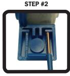
Strip wires to 5/8". Use the strip guide molded into the connector for reference.
