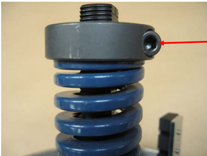
Turn the collar to increase the torque
