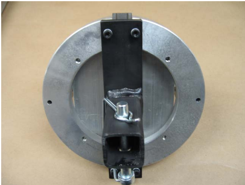
Clutch shown in the set position
