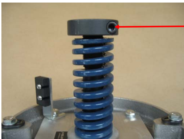
Stem has engraved graduations of 50 ft lbs increments. Side 1 shown
