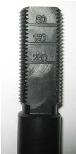
Stem has engraved graduations of 50 ft lbs increments. Side 1 shown
