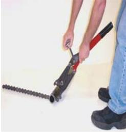
1. Place pipe on outstretched chain next to cutter jaws. Turn hand wheel counterclockwise until jaws are fully open.
