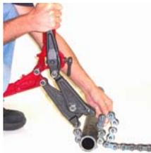
2. Holding tool in this position, wrap chain around pipe with other hand. Pull chain tight and engage the No. 16 pin nearest to the upper jaws. Be sure surplus chain comes out over the top as
