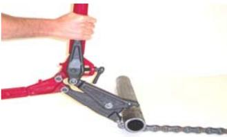
1. Place pipe to be cut on outstretched chain next to cutter jaws. Open handles to 90°, grasp cutter as shown and rest on pipe.
