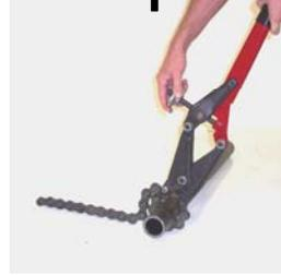
3. Rotate hand wheel clockwise to remove slack from chain.
