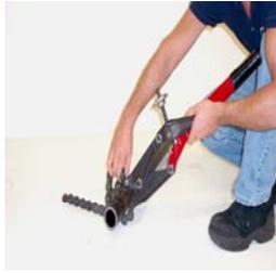
2. Wrap chain around pipe and engage nearest pin in upper jaw hooks.
