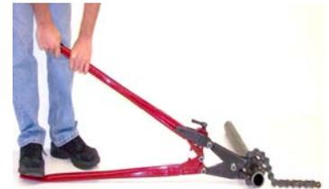
4. If you cannot achieve the proper angle with the #38 screw while the handles are closed, you have inserted the wrong pin. Disengage the chain and readjust the jaws to take the next pin. Grasp tool as shown, with one foot on lower handle and snap pipe with sharp downthrust. On extra heavy pipe, exert even downward pressure.
