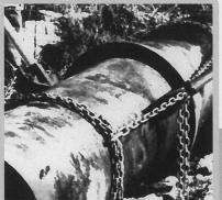
The 4012 Pipe Puller provides the answer to pulling heavy pipe and fittings into position easily.
