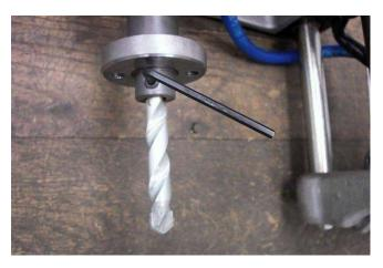
Loosen the set screw with the Allen key and insert pilot drill. Make sure pilot drill is aligned for the set screw to tighten on drill flat.
