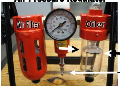
Oil Fill Line Air Pressure Adjust Knob
