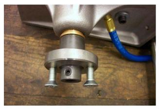
Remove the two (2) screws from the arbor.
