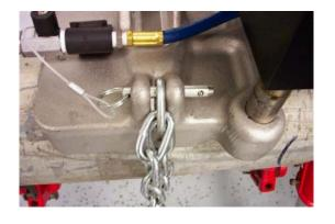
Make sure the pipe is nested properly in the saddle of the base casting. Pull chain under pipe and back to casting base. Place one chain link between casting and push pin through base and chain link. Tighten chain with hand crank.
