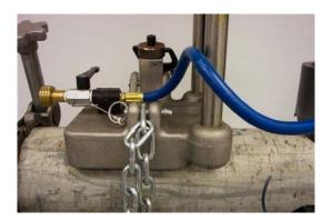
Set the hole cutter on the pipe.
