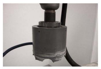
Attach the shell cutter with the two (2) screws.
