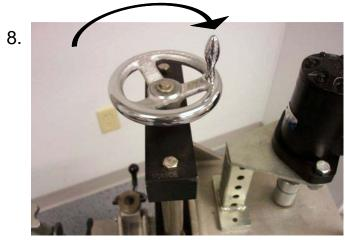
Slowly turn feed hand wheel in the clockwise position to lower the shell cutter. A heavy feed rate may damage shell cutter or pipe that is being cut. Allow shell cutter to cut material with a slow, steady turn of the feed wheel. If at anytime there are problems making the cut, stop cutting immediately.
