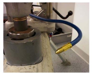
Adjust flexible hose for water stream to point on shell cutter. This is to help keep the cutter cool as well as flush away chips.
