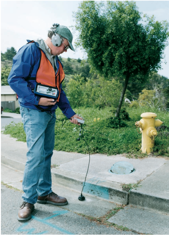
Ground Miking to pinpoint a leak in a hydrant line
