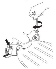
Adjust so you can easily stop the support rollers using your thumb when the blade is rotated. The support rollers should only follow the blade occasionally.
