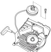
Bear in mind that the return spring lies tensioned in the starter housing. · Loosen the bolts holding the spring cassette.
