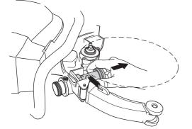
Screw the knob until it bottoms, and then loosen the knob 2 turns.
