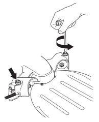
• Loosen the knob to offload the springs.
