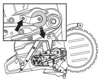
Replacing the drive belt
