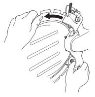
• Tighten the locking nuts on the support roller guard.
