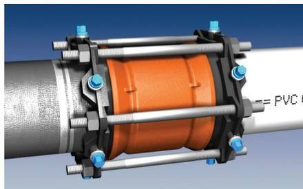
5. Hand tighten the actuating screws until all wedges are touching the pipes. Continue tightening the screws in an alternating manner until the torque limiting heads twist off. The screws may bottom out during this step.
