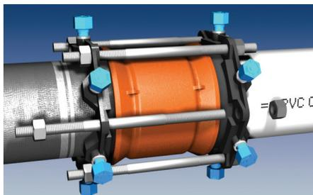
4. Install the threaded rods and hand tighten the nuts on each end. Gradually tighten the nuts in an alternating manner until the proper torque value has been reached, while maintaining the same distance between the rings and the ends of the body at all points around the rings. For 4 inch through 24 inch torque to 75 - 90 ft.-lbs., for 30 inch and greater torque to 120 - 150 ft.-lbs.
