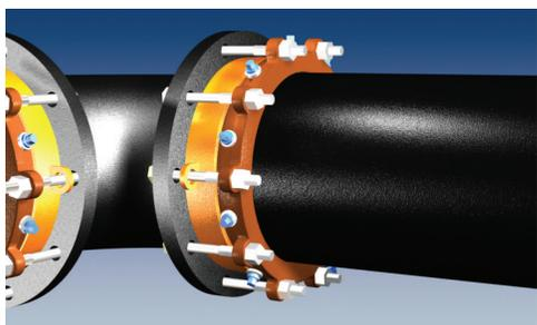
8. If removal is necessary, utilize the 5/8 inch hex head provided. For reinstallation, repeat steps 2 through 7, torquing the actuating screws to 70 ft.-lbs. or until the hex heads bottom out on the spacers or gland.
