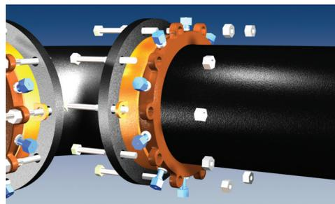
6. Insert and tighten all flange bolts. Torque all flange bolts an alternating manner to the value listed in Table 1.1. Be sure to make any necessary joint deflection before tightening the actuating screws. Joint deflection should not exceed the maximum allowable deflection. Be sure that deflection of the joint does not cause the end of the pipe to be separated from the opposing flange more than the maximum allowable gap "L".
