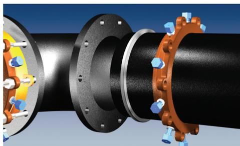
3. Lubricate and place the EBAA-Seal™ Gasket on the clean pipe following the restraint ring. (USE A TRANSITION GASKET IN PLACE OF THE EBAA-SEAL GASKET FOR CARBON STEEL AND IPS. O.D. PVC PIPE.)
